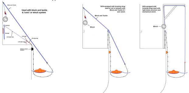
Markus MOB Scramble-net / Cradles types SCN8-200, 250, 300, 350 and 400 used with mechanical hoisting systems on FRC boat.
