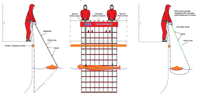
Markus MOB Scramble-net / Cradles types SCN8-200, 250, 300, 350 and 400 used manually at rail or bulwark. Applicable for workboats with rail and two deck crew.
