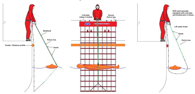
Markus MOB Scramble-net / Cradles types SCN8-200, 250, 300, 350 and 400 used manually at rail or bulwark. Applicable for workboats with rail and one deck crew.
